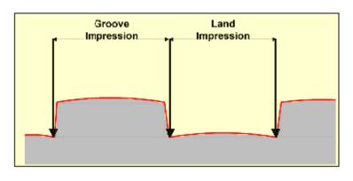
7.4.3.3.1.2 In the microscope reticle method, the fired bullet in question is mounted on a steady surface beneath the microscope. The land or groove impression of the fired bullet is positioned with both of the anchor points corresponding to points on the alignment scale. Record the measurements observed on the scale.
