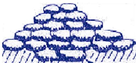
To use the pyramid method, first dig a bonding trench that will be one sack deep and two sacks wide. Place bags in this bonding layer, using this layer as the centerline for the pyramid. Next, place the sandbags to form a pyramid by alternating header courses (bags placed crosswise) and stretcher courses (bags placed lengthwise). Make sure to overlap sacks, keep staggered placement, tuck in ends and tamp into place.
